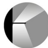
asymmetrical ceiling illumination
