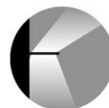
asymmetrical ceiling illumination
