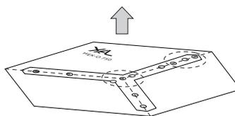
DRILL THE HOLES FOR SUSPENDED SINGLE MOUNTING
