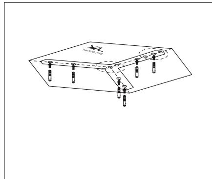
SCREW THE MOUNTING PLATE ON TO THE TEMPLATE
