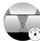
glare-free direct and 170° indirect illumination
