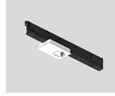
Sensor inset; SENSE (brightness, presence, temperature, humidity, air quality and noise level sensor); for lighting systems; surface traffic white; inset can be installed flexibly and without tools; flush with profile system; degree of protection IP20; PC3; 9.5-22.5V; DALI-2 control;
