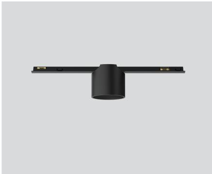
Cylindrical spotlight in aluminium; surface jet black powder coated; light inset can be installed and moved without tools by means of clip mount; power supplied via MOVE IT system track profile; hot plug protection; passive cooling of the LEDs through improved heat sink geometry; light colour 3000 K; binning initial MacAdam
