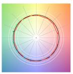
The black line represents the black body reference. The red line indicates the results of the test light source. The deviation from the test light source to the reference is shown and is marked by arrows. The shorter the arrows, the higher the color rendering.
