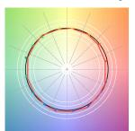
The black line represents the black body reference. The red line indicates the results of the test light source. The deviation from the test light source to the reference is shown and is marked by arrows. The shorter the arrows, the higher the color rendering.
