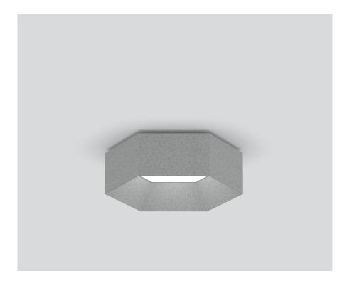
Hexagonal acoustic element made of high quality, self-supporting PET felt with sound absorbing properties, consisting of at least 50 % post-consumer recycled PET; high quality visual and tactile surface, felt grey; foreign fiber inclusions possible; to combine with HEX-O 500 or HEX-O MODULE 500; installation without tools;
