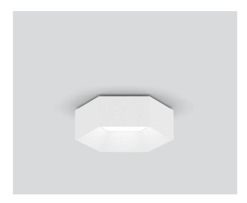
Hexagonal acoustic element made of high quality, self-supporting PET felt with sound absorbing properties, consisting of at least 50 % post-consumer recycled PET; high quality visual and tactile surface, white; foreign fiber inclusions possible; to combine with HEX-O 500 or HEX-O MODULE 500; installation without tools;
