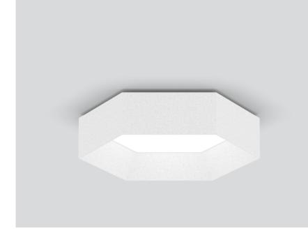
Hexagonal acoustic element made of high quality, self-supporting PET felt with sound absorbing properties, consisting of at least 50 % post-consumer recycled PET; high quality visual and tactile surface, white; foreign fiber inclusions possible; to combine with HEX-O 750, HEX-O MODULE 750 or HEX-O MODULE FLAT 750; installation without tools;
