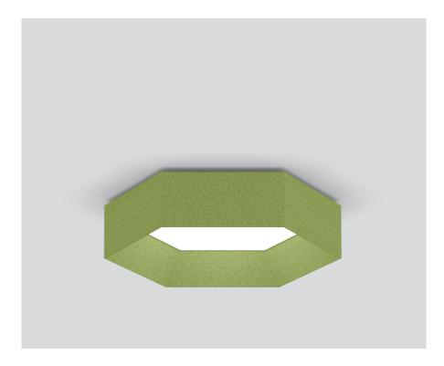
Hexagonal acoustic element made of high quality, self-supporting PET felt with sound absorbing properties, consisting of at least 50 % post-consumer recycled PET; high quality visual and tactile surface, acoustic special colours; foreign fiber inclusions possible; to combine with HEX-O 750, HEX-O MODULE 750 or HEX-O MODULE FLAT 750; installation without tools;
