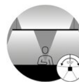
glare-free direct and 170° indirect illumination
